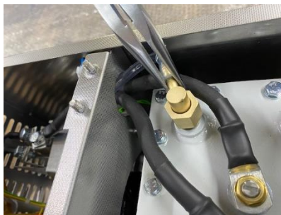
Strip off the hose using flat-nosed pliers
