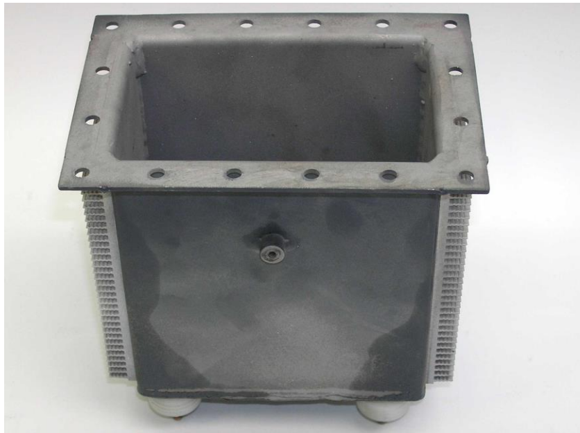
Fig. 7.5.1 Reactor opened and cleaned
