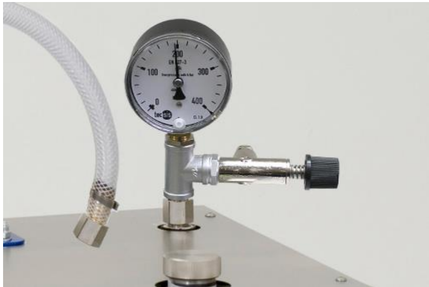
Fig. 6.1.3 Manometer mounted to gas outlet duct
