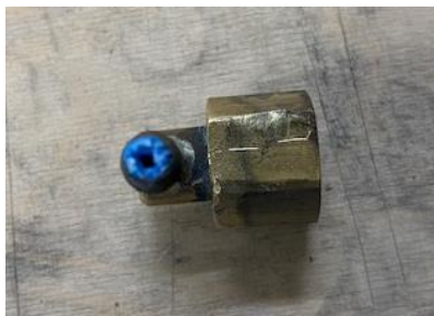
Check elbow fitting for blockage (here: blockage with blue deposit)
