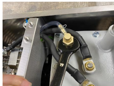
Unscrew the elbow connection with a 19mm wrench. To loosen, tap lightly against the elbow fitting.
